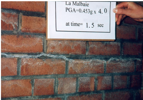
Figure 9. Pier rocking at base of central pier with Tyfo repair during La Malbaie x 4.0.
